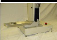
Meets ASTM D-1894 Static and Kinetic Coefficient of Friction of Plastic Film and Sheeting
